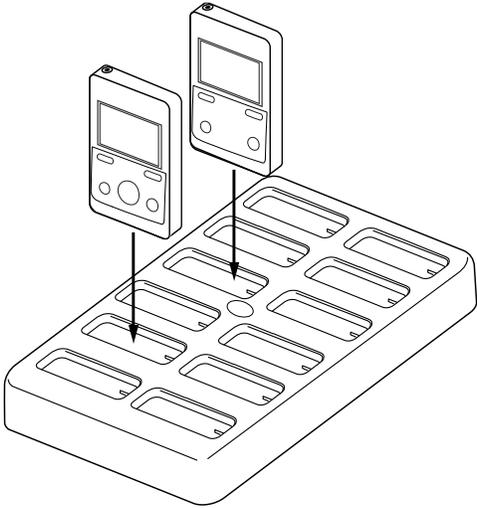
Digi-Wave DLT 400 and DLR 400 RCH can be charged in the CHG 412. 12 DLTs or DLRs can be charged at one time. The CHG 412 PRO comes with a case, but otherwise operates the same as the CHG 412.
