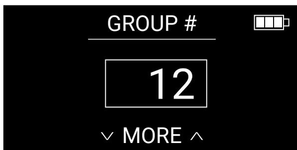
2. Join Sub-group: GUEST units are designated to exactly one sub-group. LEAD 2 units can optionally join additional sub-groups. LEAD 1 units do not have this selection as they are automatically able to join all sub-groups.
