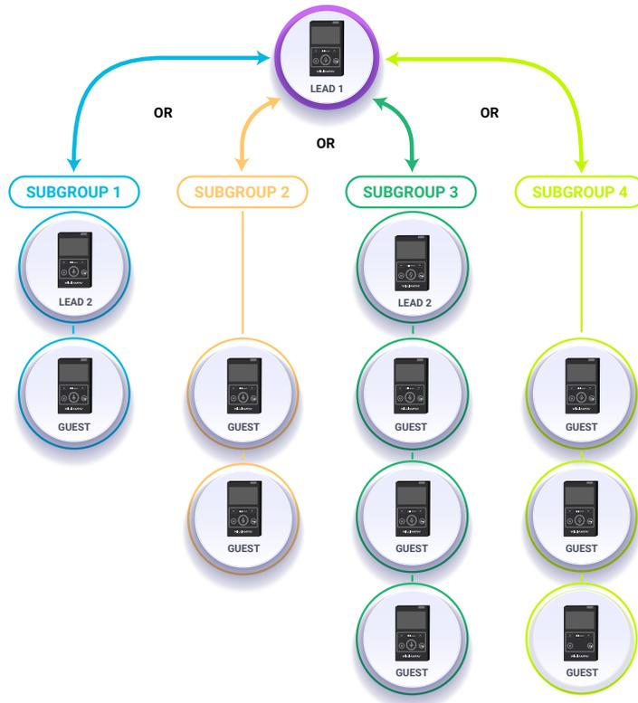
Advanced Comms mode also includes All-Call functionality. All-Call enables a Leader (LEAD 1 and optionally, LEAD 2) to pause all communication across up to 4 subgroups and address all units simultaneously.
