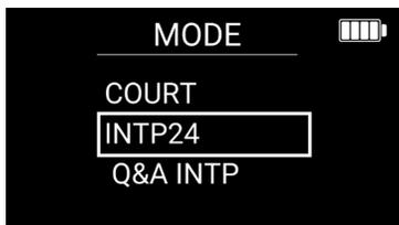
3. Make sure you choose the same mode as the MASTER unit of the Digi-Wave® system. If the modes aren't the same, then the Control unit will not be able to synchronize with the Master unit.
