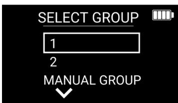
The DLR will be on channel 01. Use the arrow up button to go to channel 02-24 if desired. Hold the arrow up button to seek for active channels.
