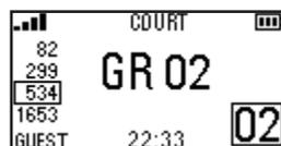
The Guest indicator will flash until the group is joined. If a device seems unable to join a group, check the PIN code.
