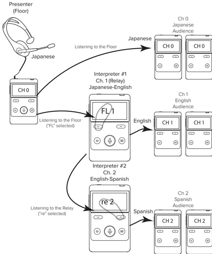
Relay Mode allows the interpreter to quickly switch between listening to the Floor on Channel 0 or the Relay on Channel 1.
