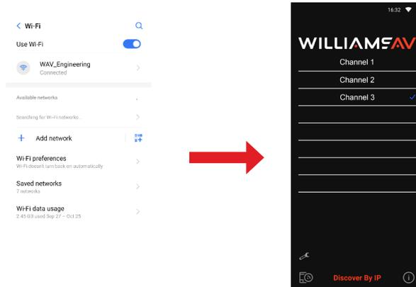
To select a different channel, push the back button and the device will re-scan the network for available channels.
