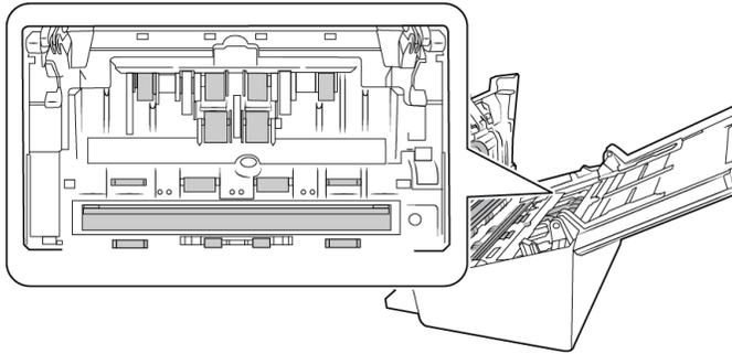
4. Wipe clean the rollers and glass in the underside of the ADF door. Rotate the rollers to clean the entire surface.
