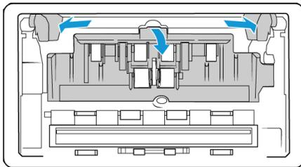
**Note:** if the paper guides are in front of the roller cover when you open it, they will automatically release from the scanner body. If this happens, follow the instructions on page 6-3 for resetting the guides in the scanner.
