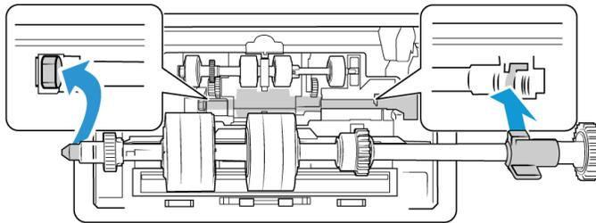
9. Rotate the locking tab into the slot in the scanner. Push on the lever until it clicks in place and locks the roller in the scanner.
