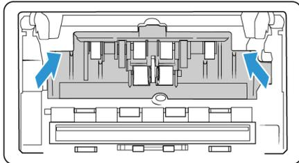
12. Make sure the paper guides are properly seated in the scanner.
