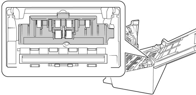
3. Move the paper guides to the side and then pull the feed roller cover away from the scanner.
