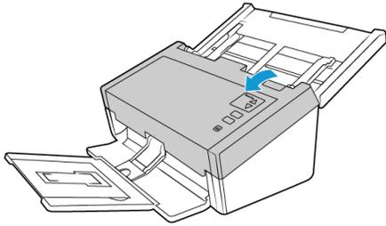
3. Wipe clean the rollers and glass in the scanner body. Rotate the rollers to clean the entire surface.
