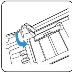
2. Gently press on the paper guide to lock the paper guide in the scanner.
