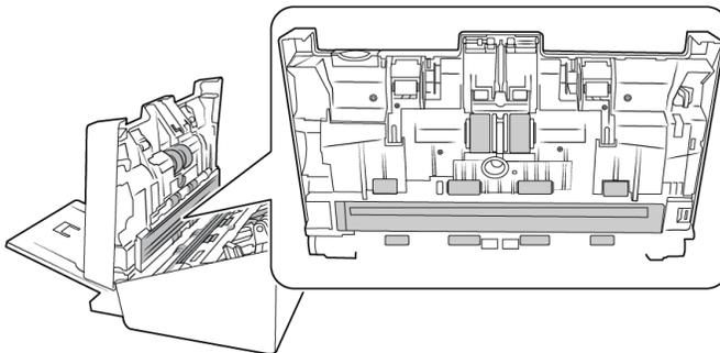
5. Using a clean, dry cotton swab, brush away any dust on the double feed detection sensors.
