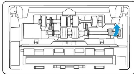
10. For the DM6440 (Scanner Part number 85-0339-### and higher) only, rotate the belt back down into place. The cover will not close if the belt is in the wrong position.
