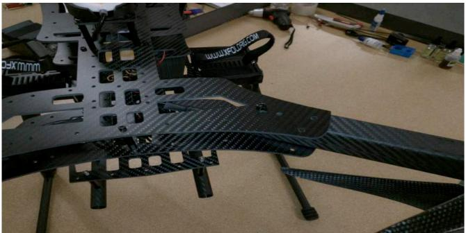
REMOVE THE 4 SCREWS AND KNOBS ALOWING THE ARMS TO SWING OUT
