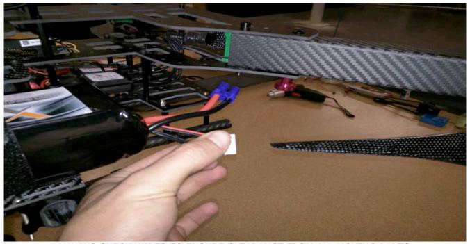
ALWAYS CHECK WIRES TO ENSURE CLEARANCE FROM ALL MOVING PARTS.
