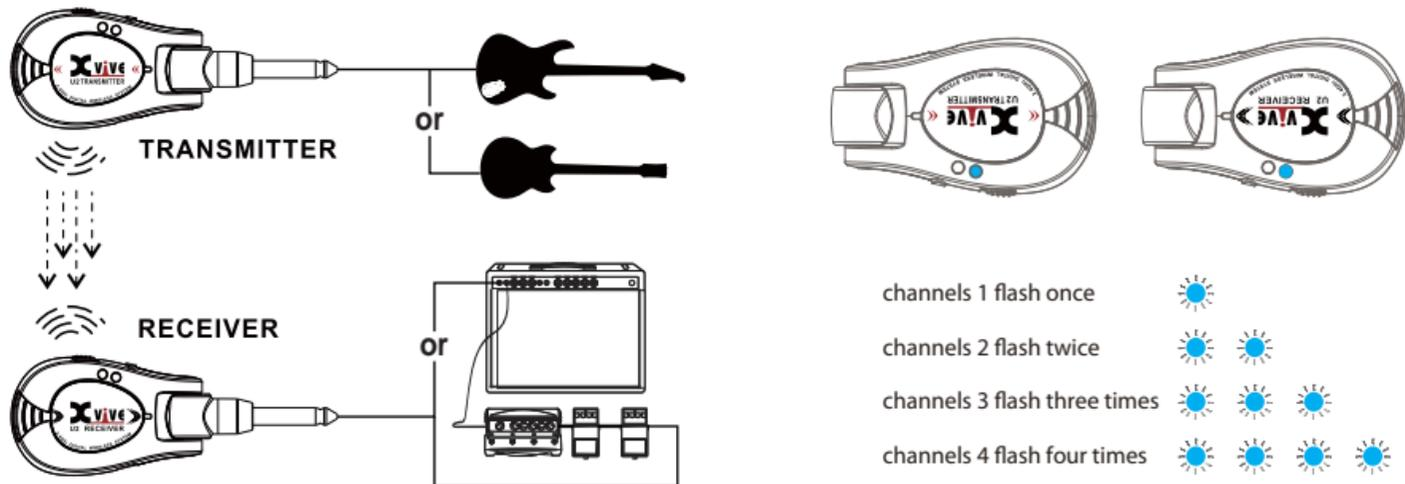
1. Transmitter plugs into the Guitar (you instruments), the receiver plugs into the effects pedal, AMP, Audio, etc.
