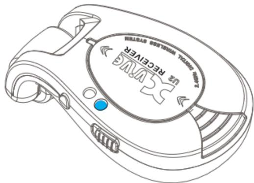
3. After connecting successfully, LED lights on receiver will keep light on.
