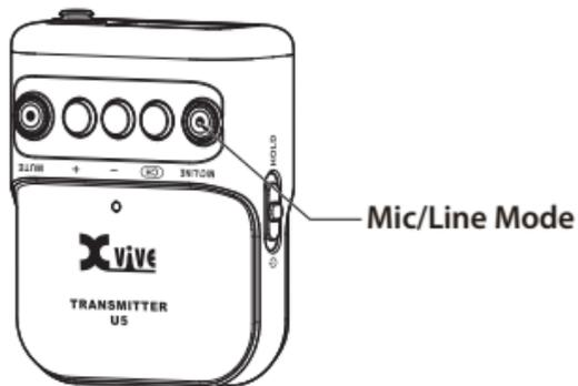
Sets the input level according to the audio input device. Choose MIC for lavalier microphone, and LINE for audio mixer or other line-level audio device.
