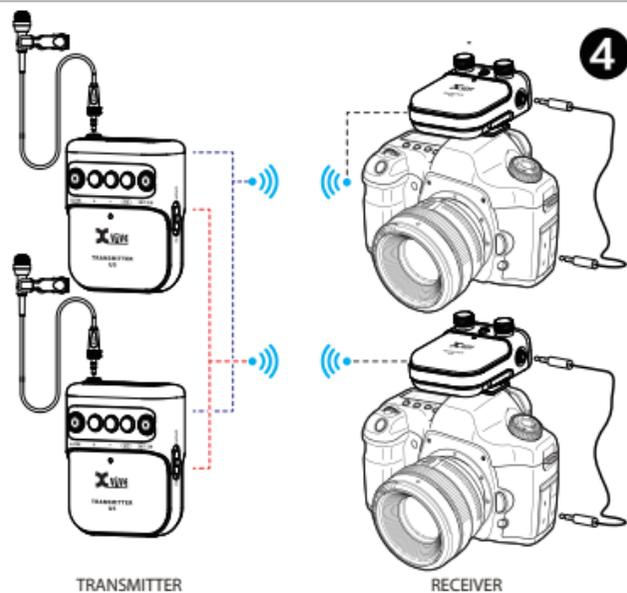
Use two receivers (set to the same channel) connected to two DSLR cameras to send them the same wireless audio.
