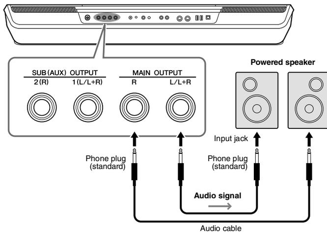
You can use the instrument's [MASTER VOLUME] dial to adjust the volume of the sound output to the external device.
