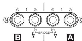
This ⚡ mark indicates a dangerous electrically live terminal. When connecting an external wire to this terminal, it is necessary either to have “a person who have received appropriate guidance on handling” make the connection or to use leads or a cord that have been manufactured in such a way that the connection can be made simply and without problem.
