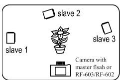
Using RX slave flash mode, effectively reduce the impact of obstructions on the radio signal, at the same time, you can get farther triggering distance, and maximum distance is up to 100 meters.
