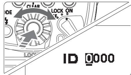
In the wireless radio transmission flash shooting process, make sure the transmission channel and ID setting of the master unit and slave unit are the same, otherwise the flash could not work normally. When the master unit and the slave unit make connection establishment, the <LINK> indicator will be in green light.
