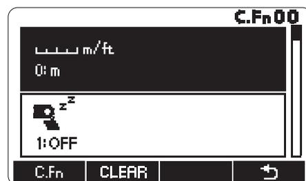
[ ]button back to the shooting interface. After entering the custom function menu,short press the function button [ **CLEAR** ], then short press the function button 1 [ **OK** ]will restore the custom function to factory default.
