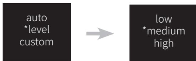
3. custom: You can customize the motor torque for three axis motors. Push the joystick up/down to select the axis motor you wish to customize and push to the right to enter the customization. In the customization, push the joystick up/down to customize the motor torque and push to the left to save the setting.
