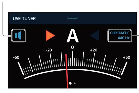
This shows the tuner type and standard pitch. Touch this to change tuner settings. (→ ["Changing tuner settings" on page 58](#))
