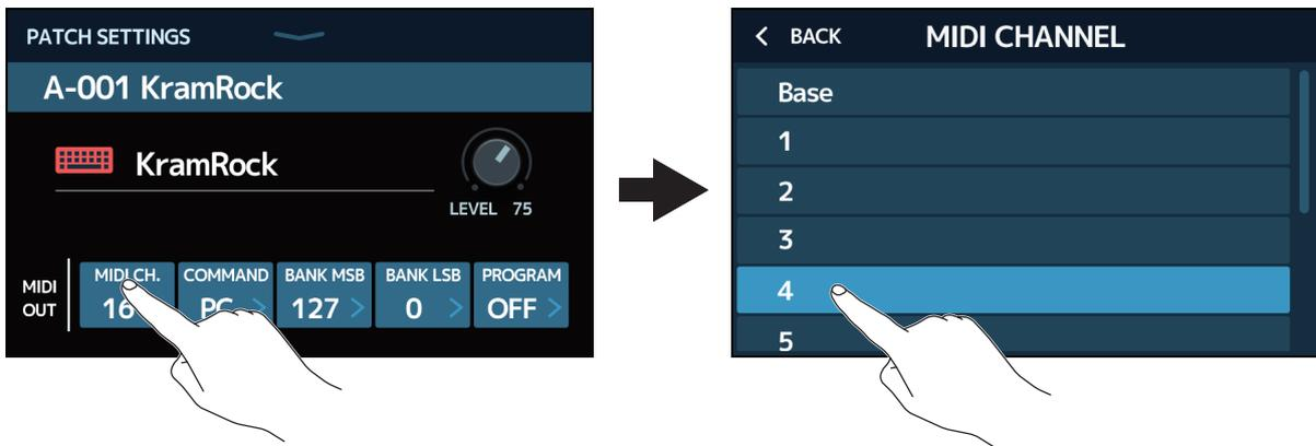
Set it to BASE to transmit on the channel set following the procedures in [“Setting the channel used to receive MIDI data” on page 83.](#)
