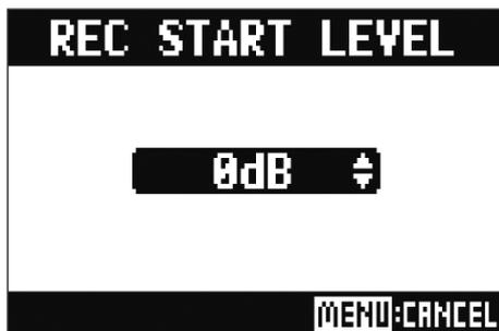
Recording will start automatically when the level of the MASTER fader output signal exceeds the set level.
