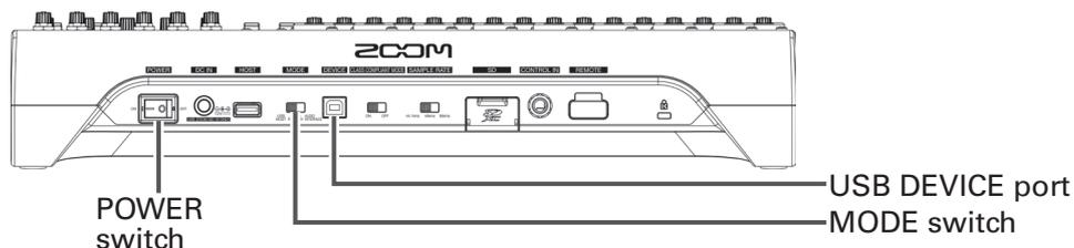
1. Use a USB cable to connect the USB DEVICE port to the computer.
