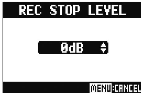
Recording will stop automatically when the level of the MASTER fader output stays below the set level for the amount of time set in step 2.
