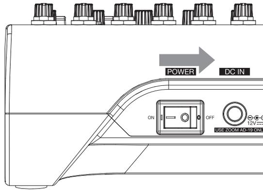
3. Plug the specified adapter (AD-19) into an outlet.
