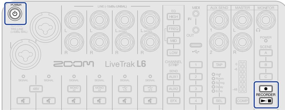
1. With the power off, insert the microSD card. (→ [Inserting microSD cards](#))
