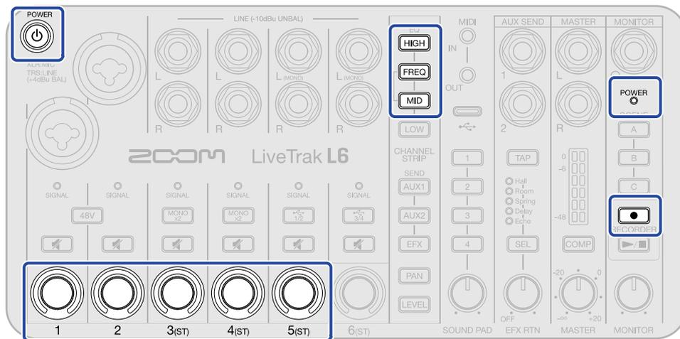
1. While pressing the **HIGH** (HIGH) and **FREQ** (FREQ) buttons, press the **POWER** button to turn on the L6 power.
