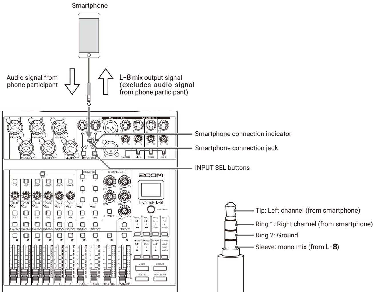
**1.** Connect a smartphone to the smartphone connection jack on the **L-8**.
