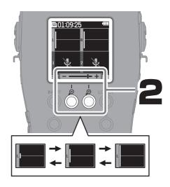
The M4 uses 32-bit float format, which can record with the same resolution for any volume level, so adjusting the recording level is unnecessary. During playback, the top and bottom edges of the waveform screen are the highest volume levels.
