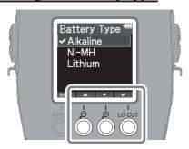
Set the type of battery used correctly so that the amount of remaining battery charge can be shown accurately.
