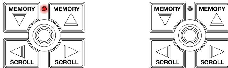
The On/Off indicator lights when the effect is on.
